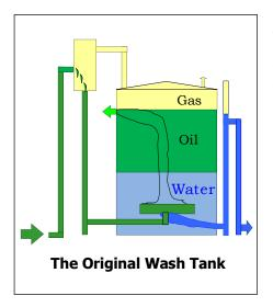
A water leg is installed on the outside of the tank. Its spillover elevation is set so the lower one-third of the tank is filled with produced water and the remainder of the tank fills with oil. As flow from oilwells begins, the spreader distributes the produced fluids into the water phase. Solids and emulsions (aka: BS&W) separate from the oil. Separated water is absorbed into the water layer and solids settle onto the bottom of the tank.
