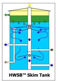
the entire cross section of the tank. At this point, the water has slowed to its slowest downward velocity so all separable oil droplets can counterflow upward and into the oil layer above. This uniform and efficient fluid distribution maximizes retention time and assures efficient and near-total oil-water separation.
