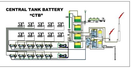
From 2014 point on every new CTB was constructed according to a master design like the one sketched at the left.
