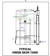
outlined a radical innovative design correcting the flow deficiencies of the gunbarrel in the more dominant high water cut applications of the day. This patented design was identified by the acronym HWSB® (hydro-dynamic water separation breakthrough). Its original patent was improved upon and was subsequently through the first two decades in the 21st century. The gunbarrel tank's water retention time of 35 seconds increased to 45
