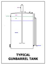
with a vertical pipe down through the center of its tank as shown in the graphic at the left. This pipe, referred to as the "downcomer," is the conduit that sends the incoming mix of water and oil (emulsion) into the tank. The downcomer pipe extends through the roof of the tank and ends inside the tank near its bottom. The produced fluids enter the downcomer pipe near its top.
